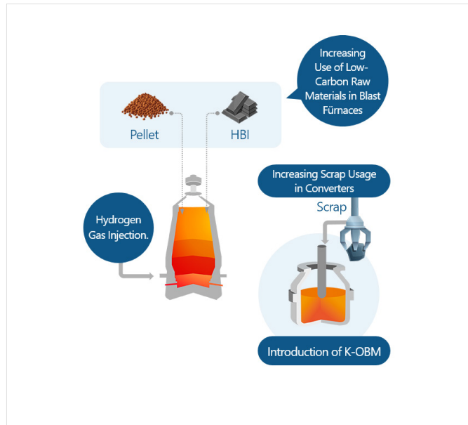
Key Bridge Technologies Based on Blast Furnace/Converter
